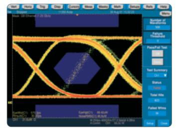
**Figure 5.** Eye diagram showing faulty bit.
