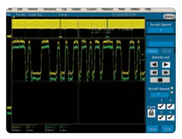
Figure 10. Two locked zoom regions being automatically scrolled.
